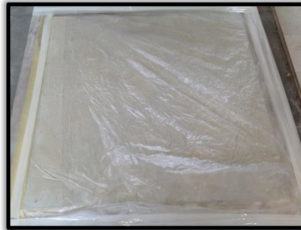
Apply the tape on the borders of the plastic film.
